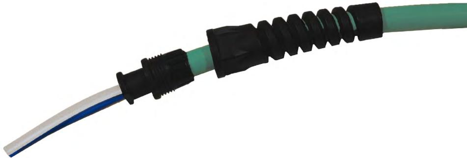
5. Put special glue for plastics materials on the screw thread of the top part of the spring. Move the anti-kink spring up along the hose and screw it around the top part. Your hose is ready for use.
