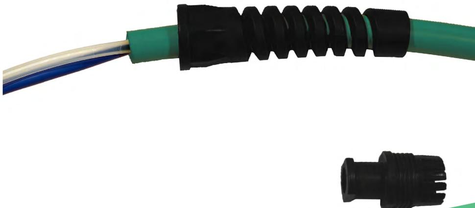
3. Put the rubber seal at the end of the hose with a margin of 3mm (see below).
